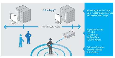
The terminals supplied to warehouse operators receive the data directly from Click Reply™ WM module and translate them into voice commands; the operators' answers are then digitalized and readdressed to the system in real-time.
