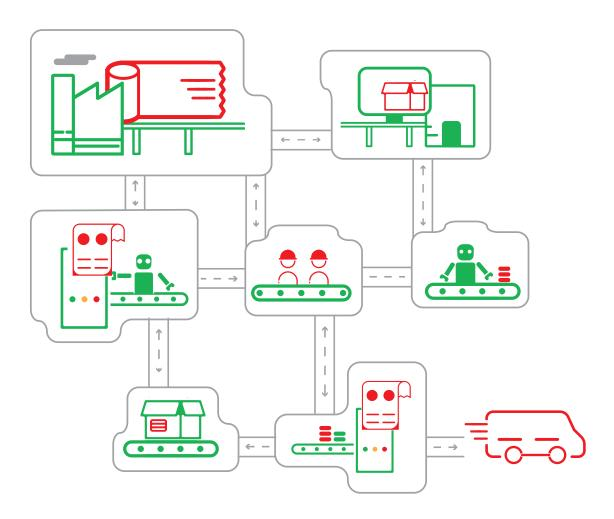
Autonomous assembly islands are stations along the production cycles of industrial products, where manufacturing operations are performed independently from the assembly line. Products to be manufactured or assembled are transported to these islands (or cells) where workers perform the necessary tasks – with or without the support of industrial robots.
